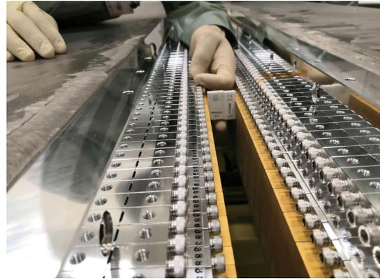
Fig. 8 (Color online) A photograph of the new magnet-array for the IR-undulator during the installation into the FEL-beam-line.
