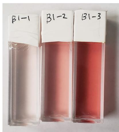
Fig. 14 (Color online) Gel dosimeters after radiation exposure in the accelerator room. The red-color concentration of the dosimeters depends linearly on the absorbed dose.
