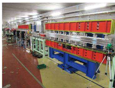
Fig. 3 (Color online) Design of the undulator for MIR-FEL (Left) and photograph of two undulators installed in the south-straight section of the cERL (Right).
