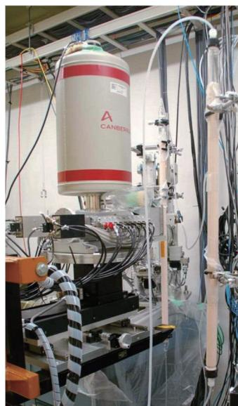
Fig. 9 Layout of XAFS measurement of the ion exchange process.
