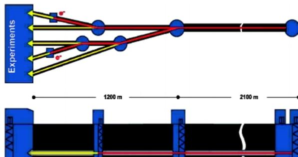
Fig. 3 Schematic Layout of the underground tunnel system of the European XFEL Facility in Hamburg.
