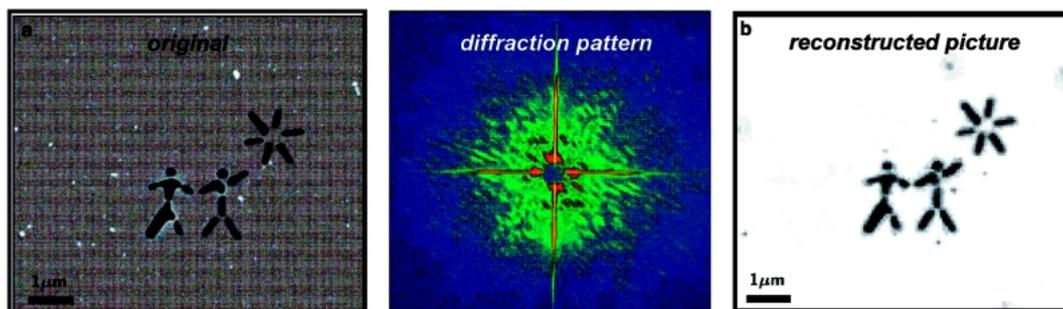
Fig. 11 Single shot diffraction pattern taken with 32 nm FEL radiation from FLASH and reconstruction.
