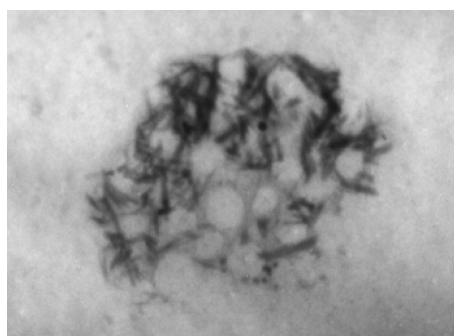
Fig. 3 X-ray imaging photo of the simulated glass obtained at 22.2 keV. The aggregation of needle-like \text{RuO}_2 solid is observed as a cage form.
