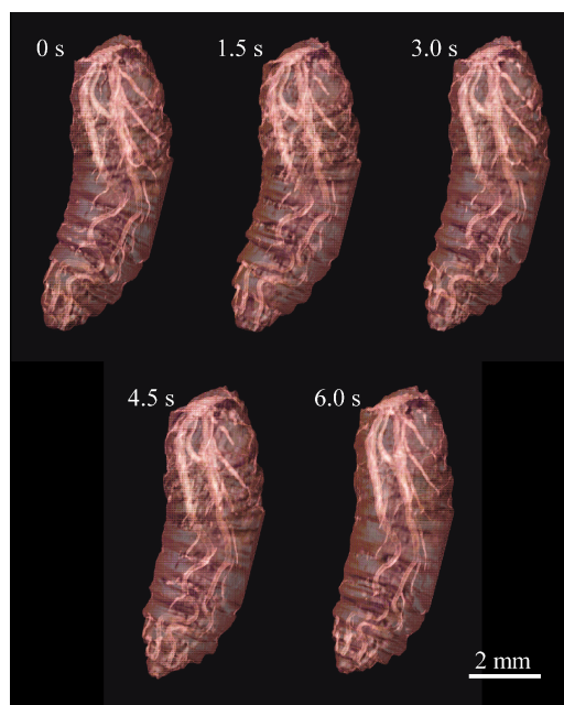
Fig. 10 Series of phase tomograms of a living red maggot (fishing worm) obtained with Talbot interferometry and white synchrotron radiation.
