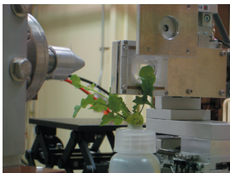
Fig. 4 A photo of in vivo XRF analysis of A. halleri (Spring-8 BL37XU).
