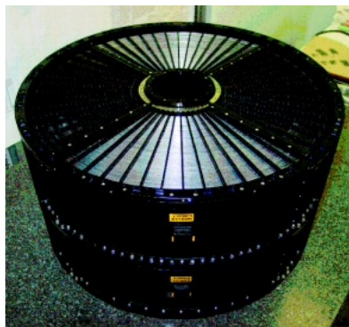
Fig. 3 X-ray telescope (XRT) of 40 cm in diameter.
