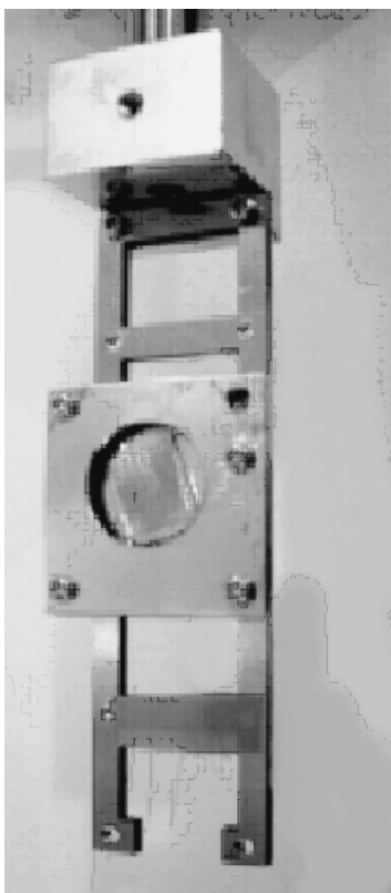
Fig. 6 Sample holder for the liquid specimen with using PVDC membrane.
