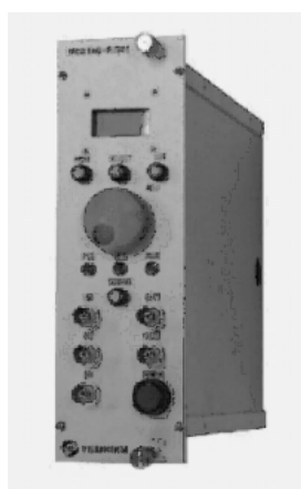
Figure 5. A MOSTAB module developed at SPring-8. This NIM 2 unit module includes a DSP and a microprocessor which is remote-controllable through an Ethernet using the TCP/IP protocol. The module was designed and manufactured by TEIKOKU DENKI SEISAKUJO Co., Ltd.
