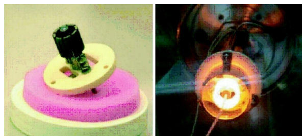
Figure 7. Cathode assembly (left). The \text{CeB}_6 single crystal cathode (3 mm diameter) is mounted on the high-purity graphite rod. The cathode is heated up to 1400 degree C using graphite heater (right).
