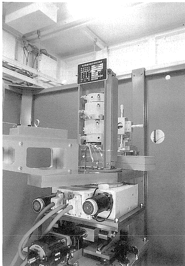
Figure 7. High-pressure gas vessel with an x-ray diffractometer installed at BL04B1 beamline.
