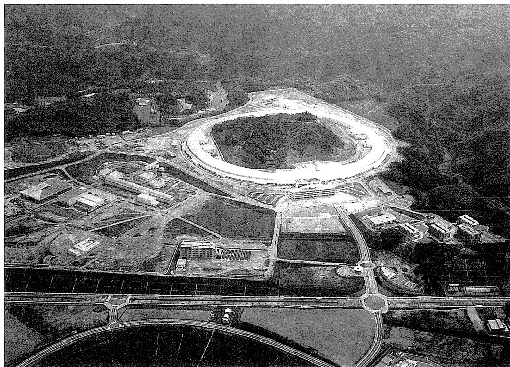
Figure 1. An aerial view of the SPring-8 facility. The storage ring is built around a hill. The injectors are built at the level 10 m below the level of the storage ring.
